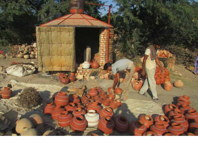
**Earthen Crafts:** Promotion of Energy efficient kiln for terracotta products and motorized tools like electric potter's wheel and pug mill for production and energy efficiency.
